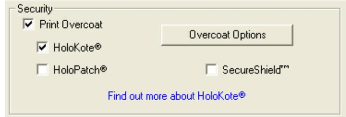
When **Print Overcoat** is **enabled**, the areas of the card that are protected by overcoat can be configured by clicking on the **'Overcoat Options'** button.
