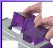
2. Tilt the loaded hopper back as shown, and lower gently into the receptacle at the rear of the printer. You will be able to lower the hopper about an inch (25mm).
